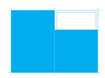
4 Page False Cover Front: 297mm W x 320mm H Back: 297mm W x 420mm H Bleed: 4mm on all edges Marks: Crop marks
