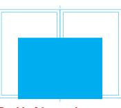
**Double A4 spread** Trim: 383mm W x 240mm H Copy: 377mm W x 234mm H **Bleed:** 389mm W x 246mm H
